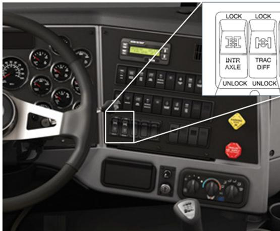
Figure 3: In-cab Differential Lock Switch
