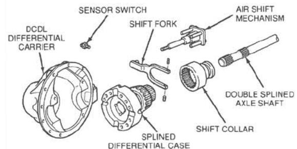
Figure 2: DCDL consists of 7 unique components
