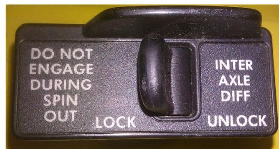
Figure 5: Typical IAD switch
